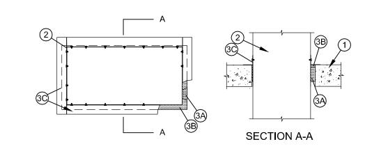
1. Floor - Min 4-1/2 in. (114 mm) thick reinforced lightweight or normal weight (100-150 pcf or 1600-2400 kg/m3) concrete floor.
