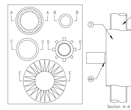
1. Floor Assembly – Min. 4-1/2 in. thick reinforced lightweight or normal weight (100-150 pcf) concrete. 2. Firestop system — The firestop system consists of any combination of the four individual firestop configurations described
