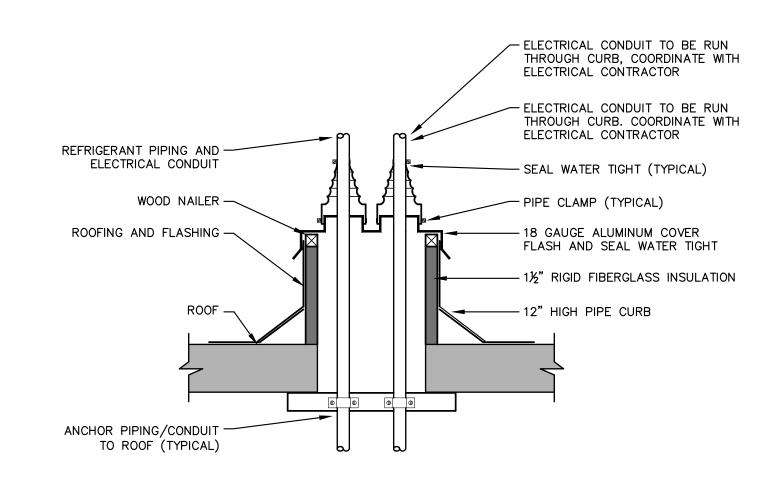
1. HVAC CONTRACTOR SHALL COORDINATE ALL CURB AND PENETRATION FLASHING REQUIREMENTS WITH THE GENERAL CONTRACTOR. ALL PENETRATIONS SHALL BE SEALED AIR AND WATER TIGHT.
