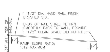
LRAMP, SEE NOTE BELOW. 1. RAMP SURFACES SHALL BE FINISHED WITH NON-SKID SURFACE AND SHALL BE A MINIMUM WIDTH OF 36". ALL RAMPS AND RAILS SHALL COMPLY WITH ALL RULES AND REGULATIONS OF THE LOCAL, STATE AND ALL OTHER APPLICABLE CODE.
