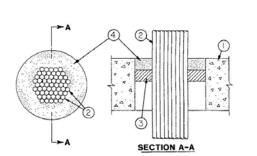
1. Floor or Wall Assembly — Min 4-1/2 in. (114 mm) thick lightweight or normal weight (100-150 pcf or 1600-2400 kg/m3) concrete. Wall may also be constructed of any UL Classified Concrete Blocks\*. Max diam of opening is 6-1/4 in. (159 mm). See Concrete Blocks\* (CAZT) category in the Fire Resistance Directory for names of manufacturers.
