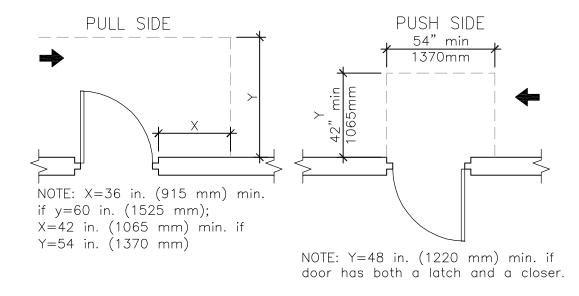
HINGE SIDE APPROACHES - SWINGING DOORS NOTE: All doors in alcoves shall comply with clearances for front approaches.
