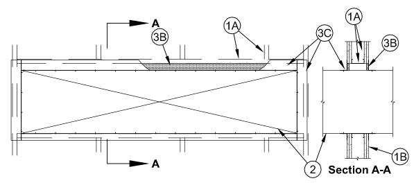
1. Wall Assembly - The 1 or 2 hr fire-rated gypsum wallboard/stud wall assembly shall be constructed of the materials and in the manner described in the individual U400 or V400 Series Wall or Partition Design in the UL Fire Resistance Directory and shall include the following construction features: A. Studs - Wall framing shall consist of min 3-1/2 in. (89 mm) wide steel channel studs spaced max 24 in. (610 mm) OC. Additional steel studs shall be used to completely
