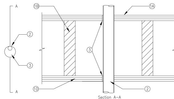
1. Floor- Ceiling Assembly - The 1 hr fire-rated joist floor-ceiling assembly. The general construction features of the floor-ceiling assembly summarized below:
