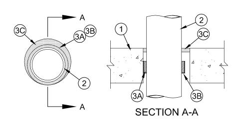
1. Floor Assembly — Min 4-1/2 in. (114 mm) thick reinforced lightweight or normal weight (100-150 pcf or 1600-2400 kg/m3) concrete. Max diam of opening is 6 in. (152 mm).
