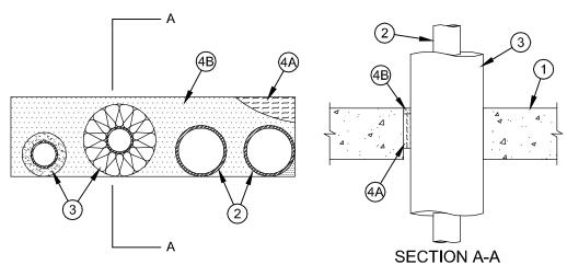
1. Floor or Wall Assembly - Min 4-1/2 in. (114 mm) thick reinforced lightweight or normal weight (100-150 pcf or 1600-2400 kg/m3) concrete floor or min 5 in. (127 mm) thick reinforced lightweight or normal weight concrete wall. Wall may also be constructed of any UL Classified Concrete Blocks\*. Max area of opening is 168 in.2 (1084 cm2) with max dimension of 24 in. (610 mm). See Concrete Block (CAZT) category in the Fire Resistance Directory for names of manufacturers.
