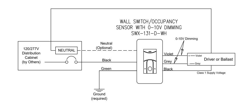
WALL SWITCH / OCCUPANCY SENSOR W/DIMMING
