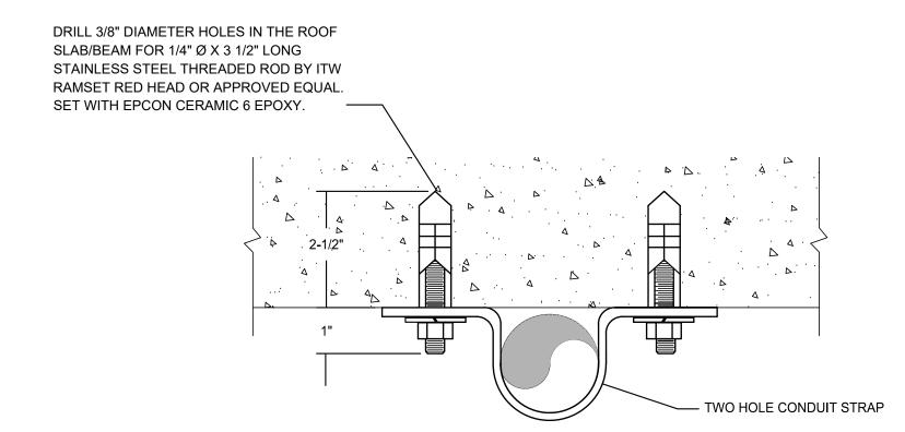
6 CONDUIT MOUNTING FOR HORIZONTAL SURFACES
