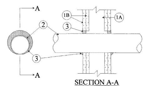
1. Wall Assembly —The 1 or 2 hr fire rated gypsum wallboard/stud wall assembly shall be constructed of the materials and in the manner described in the individual U300 or U400 Series Wall or Partition Design in the UL Fire Resistance Directory and shall include the following
