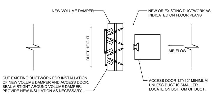
CUT EXISTING DUCTWORK FOR INSTALLATION OF NEW VOLUME DAMPER AND ACCESS DOOR.
